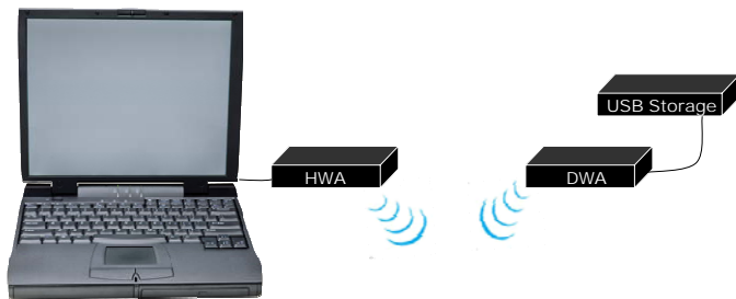
Figure 7: W-USB test configuration Throughput of W-USB products was measured by timing the file transfer via the W-USB link between the host wireless adapter (HWA) and the device wireless adapter (DWA).
