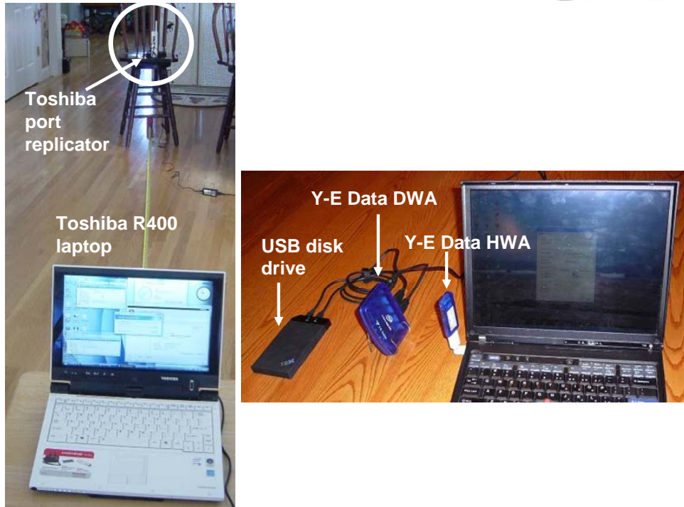
Figure 12: Photos of test setups – left: Toshiba laptop and its port replicator ; right: Y-E Data W-USB test setup with the USB drive used to copy the file. The Toshiba port replicator data ports were tested without the display connected since the display drastically limited the range of operation.
