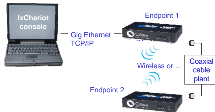
Figure 10: CWave test setup for measuring TCP/IP throughput with the IxChariot
