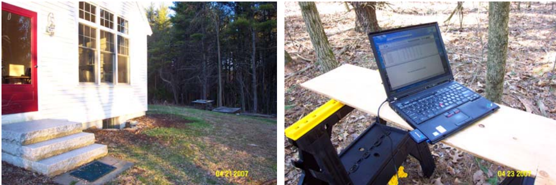
Figure 7: Home setting – outdoors locations. The AP was located behind the window in the exercise room (left) with outdoor locations in the woods (right) slightly downhill from the house. Plastic supports were used with a wooden top to hold the client PC.
